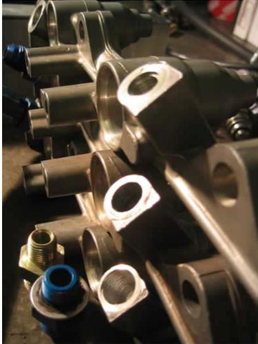
The 12 mm hole is the one on the bottom and the stock rail is the one on the top. The M12 fitting (blue one) is show next to the 1/8" npt fitting in the bottom left corner of the picture.
