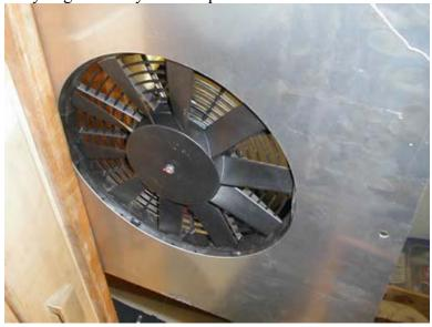
Hold the fan in place and mark the holes with a pen or a punch. Do this for both fans. Now, drill the 4 ¼" holes for each fan. Use a small pilot bit first to help you keep the holes from wandering when you start them. Now, using the spacers, long 10-32 screws, washers, lock washers, and nuts flip each fan over and screw it in place using the spacers to put it at the correct height.
