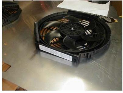
Remove the punch and drill the holes. Use a smaller drill first as a "pilot drill" and then run a ½" bit in. Now, use the 8 1 ½" long 10-32 screws with washers, lockwashers, and nuts and mount the fans as shown above and you are done!
