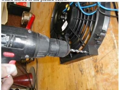
These holes will be used to hold the fans in. Now lay each fan as it will be mounted and use a punch or pen to mark the 4 holes for each fan.
